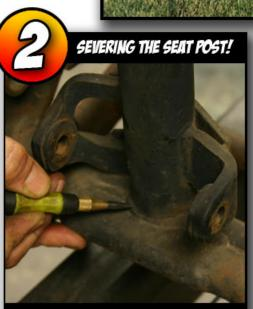
SEVER THE SEAT POST AS FAR BELOW THE REAR MOTOR MOUNT AS POSSIBLE... THEN... SAND THE OUTSIDE FOR WELDING AND EVICT ALL RODENTS AND INSECTS LIVING WITHIN.
