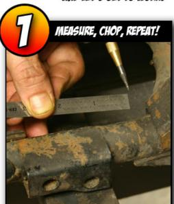
1" BEHIND THE EXHAUST MOUNTS, MARK AND CUT THE LOWER FRAME RAILS. AFTERWARDS, CLEAN THE 1" SECTION OF FRAME AND DRILL A 3/8" MIN. HOLE THROUGH THE BOTTOM ONLY!
