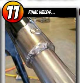
NOW THAT EVERYTHING IS TACKED IN PLACE AND ALIGNED, FINAL WELDS MAY BE APPLIED INCLUDING THE SLUG HOLES AT EACH REAIL CONNECTION.
