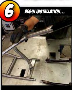
INITIALLY INSTALL YOUR HARDTAIL BEGINNING WITH THE BACKBONE AND MANIPULATE THE LOWER SLUGS INTO THE FRAME RAILS
