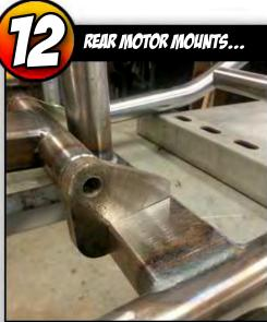
MOCK YOUR MOTOR IN PLACE AND BOLT THE TWO MOTOR MOUNTS TO THE LOWER REAR ENGINE.
