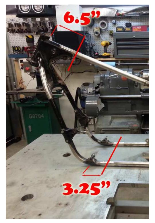
Clean inside and outside the cuts and drill a plug hole as shown:
