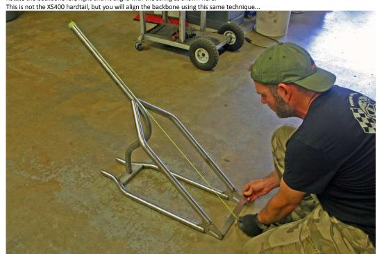
To install, slide the lower rails of your XS400 frame 2 inches INSIDE the hardtail like this...
