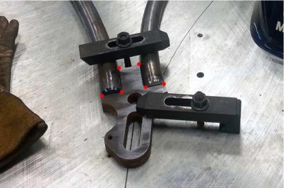
When both sides have been tacked, prop them up mirroring each other with the seat stay, chain stay, and rectangular cross tube in place.
