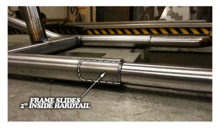
And splice the new backbone to the old using the provided slug.
