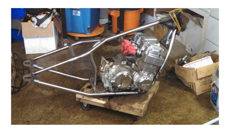
I'm sure you noticed that the upper cross bar (seat stay) was simply tacked in place when we shipped it to you. This is so that you can cut the tacks, and position the seat stay according to the size and design of your seat and springs (if any).
