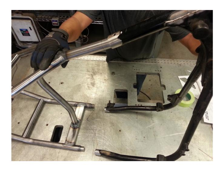
Once the hardtail is in place, you will check the alignment of the hardtail to the factory frame. Do this by securing a string to the very top dead center of your frame's head tube. Using a ruler, find the center point between your axle plates. Run the string from your head tube to the center point between the axle plates and adjust the hardtail left or right until the string becomes aligned with both the factory frame and the backbone of the hardtail as shown:
