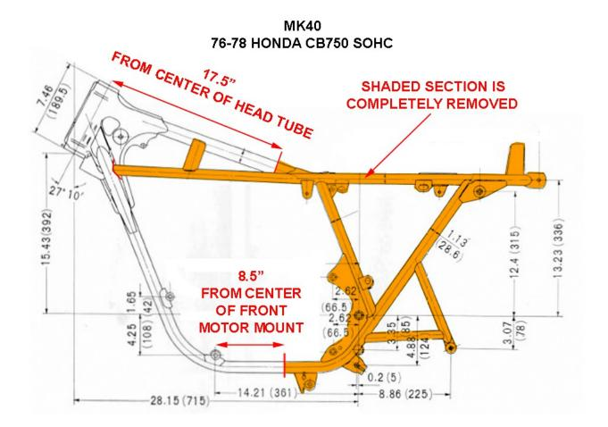
Once your cuts are complete, you will need to prepare the surfaces for welding. Begin by cleaning around the OUTSIDE and INSIDE of your cuts with sand paper or a Dremel type tool. Drill a small hole (around 1/4") no more than 1 inch away from the cut line. This will be used to weld a slug anchor once the hardtail is installed. Repeat the process on the lower two rails as well...
