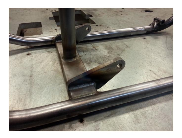
As a precaution... We suggest placing a washer BETWEEN the motor mount plates and the motor before tacking the mounts in place. Once the mounts are tack-welded in place, remove your motor and apply full welds to the mounts inside and out.
