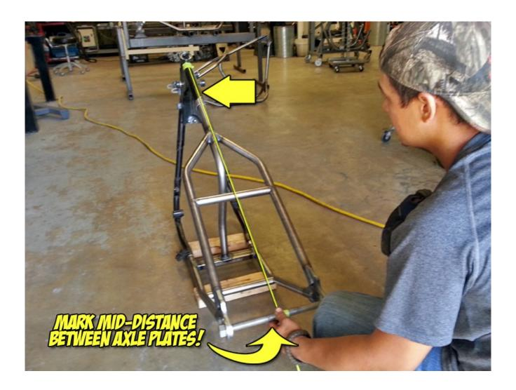
After aligning the backbone, make sure that the axle plates are 90 degrees horizontal to the frame. This does not require laser technology... Just use your good "eye" and verify that your rear wheel will mount straight up and down and not angled to one side or the other...
