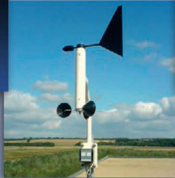
Wind Speed & Direction Sensors UKAS calibrated
