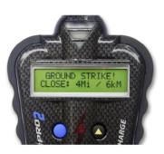
Tracks dangerous thunderstorm activity from over 130 miles. Large backlit LCD display with multiple storm status updates including. Automatically displays in both Miles and Kilometers.
