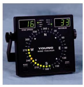
Wind direction information is clearly displayed on a circular compass pattern of LEDs. Multicolored segments give a quick visual indication of current direction and direction variability. Front panel brightness control allows adjustment for best viewing in any light.
