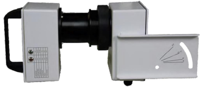
ALS-2 Calibrator connected to the ALS-2 for in situ calibration
