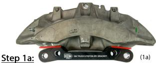
Mark, then Grind inner caliper lobes flat. Perpendicular to fit bracket as pictured in red (1a), remove material until flat with existing mating surface.
