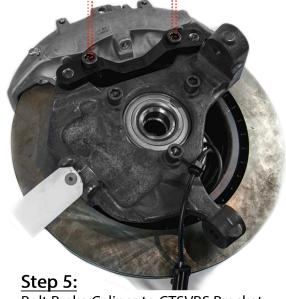
Bolt Brake Caliper to CTSVBS Bracket.
