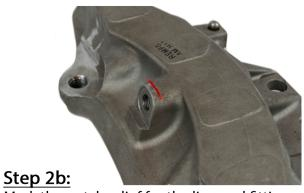
Mark the notch relief for the line end fitting...
