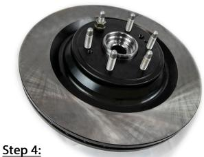
Install Brake Rotor to Hub Assembly.
