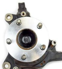
5. Get your ROTOR SPACER and make sure the CHAMFERED EDGE (logo side) is facing TOWARD the HUB SURFACE.
