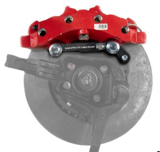
8. Next, place the CALIPER on the BRACKET with the BLEEDERS facing up.
