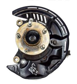
1. First, start by removing your stock CALIPER and ROTOR until you are all the way down to the HUB, as shown in this picture.
