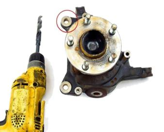
4. For this next step, you will need a DRILL and a 9/16" DRILL BIT. You will need to drill out the TOP caliper mounting hole, so that it can accept the larger 14mm bolt that the C6 Z06 CALIPER requires.
