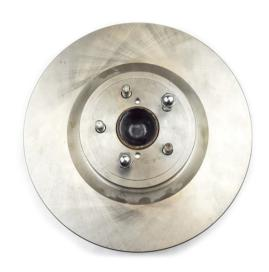
6. Thread Bolt into SPACER, but don't fully tighten. Next place the ROTOR on top of the spacer and screw on two lugnuts, to keep rotor secure.
