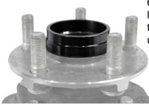
6. Carefully install HUB EXTENDER by lining up evenly with HUB SURFACE, lightly tap on the HUB EXTENDER with a hammer until it is fully seated.
