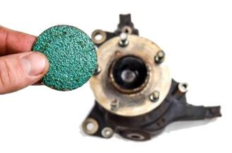
3. Remove Stock WHEEL STUDS. Take some sandpaper, or an abrasive pad, and clean any debris or corrosion off of the HUB's SURFACE.
