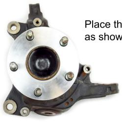
Place the SPACER down on the HUB as shown here.
