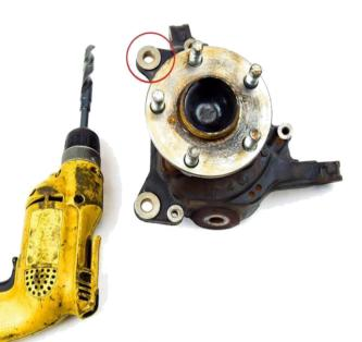
4. For this next step, you will need a DRILL and a 9/16" DRILL BIT. You will need to drill out the TOP caliper mounting hole, so that it can accept the larger 14mm bolt that the ATS CALIPER requires.
