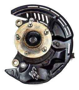
1. First, start by removing your stock CALIPER and ROTOR until you are all the way down to the HUB, as shown in this picture.
