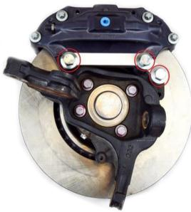
8. Next, place the CALIPER on the BRACKET with the BLEEDERS facing up.
