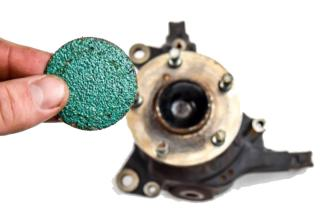
3. Take some sandpaper, or an abrasive pad, and clean any debris or corrosion off of the HUB's SURFACE.
