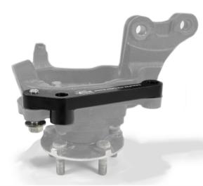
7. Place the BRACKET on the back of the SPINDLE with the raised section FACING the ROTOR as shown.
