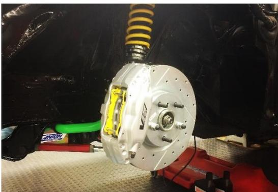
Now install the pads, pins, and clips just as you would on a CTS-V. You can also attach your brake lines now. (300zx's require banjo bolt style 240sx lines)
