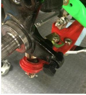
Take the provided M14 x 2.0 tap and tap the BOTTOM caliper bolt hole that is closest to the ground. Be very careful to make sure the tap goes in straight or the bracket will not line up properly. After you completed tapping the hole insert one of the M14 bolts to ensure the bolt fits properly.
