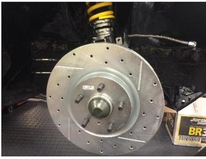
Now that you have fitted the caliper and bracket to the knuckle properly, remove them and install the 350z 12.75" rotor. Hand tighten 2 or 3 lug nuts to help keep the rotor in place.
