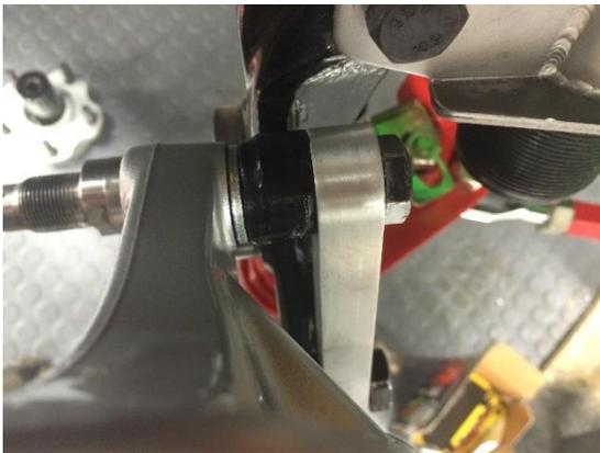
Before bolting the caliper on make sure to take one of the M12 washers and put it on the top bolt between the caliper and knuckle. Now hand tighten the two M12 bolts onto the caliper. Once the caliper is snug against the bracket and knuckle you can torque down the M14 bolt first then the two M12 bolts.
