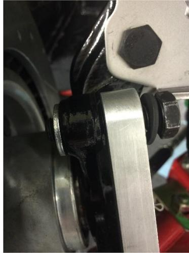
Next take the M14 bolt and start to thread the bracket onto your knuckle. Only hand tighten it, do not torque it down yet. Also slide in two of the M12 bolts into the other holes. Make sure there are washers between the bolt head and bracket.
