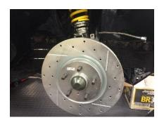
Now that you have fitted the caliper and bracket to the knuckle properly, remove them and install the 370z 14" rotor. Hand tighten 2 or 3 lug nuts to help keep the rotor in place.
