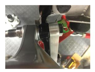
Before bolting the caliper on make sure to take one of the washers and put it on the top bolt between the caliper and knuckle. Now hand tighten the top and bottom bolts onto the caliper. Once the caliper is snug against the bracket and knuckle you can torque down the center bolt first followed by the top and bottom bolts.
