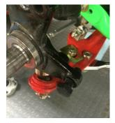
Take the provided M14 x 2.0 tap and tap the BOTTOM caliper bolt hole that is closest to the ground. Be very careful to make sure the tap goes in straight or the bracket will not line up properly. After you completed tapping the hole insert one of the M14 bolts to ensure the bolt fits properly. After tapping the bottom hole drill out the TOP caliper bolt hole with a 9/16" drill bit to accept the larger M14 bolt.
