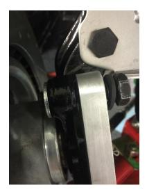
Next take the center M14 bolt and start to thread the bracket onto your knuckle. Only hand tighten it, do not torque it down yet. Also slide in the other two M14 bolts into the remaining holes. Make sure there are washers between the bolt head and bracket.
