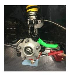
Begin by removing your existing brake caliper, rotor, and brake line. You should be all the way down to you hub.
