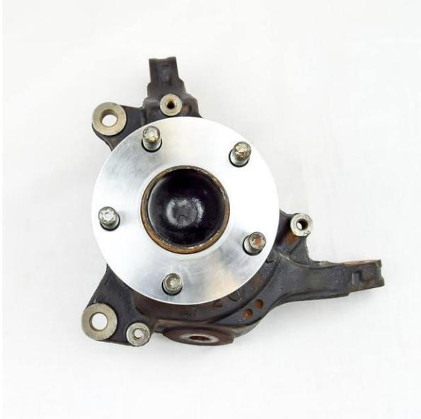
Place the spacer down on the hub as shown.
