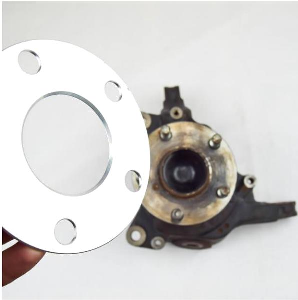
Next grab your rotor spacer and make sure the chamfered edge is facing towards the hub surface.
