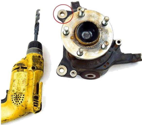
For this next step you will need a drill and a 9/16" drill bit. You will need to drill out the top caliper mounting hole to accept the larger 14mm bolt that the ATS caliper requires.
