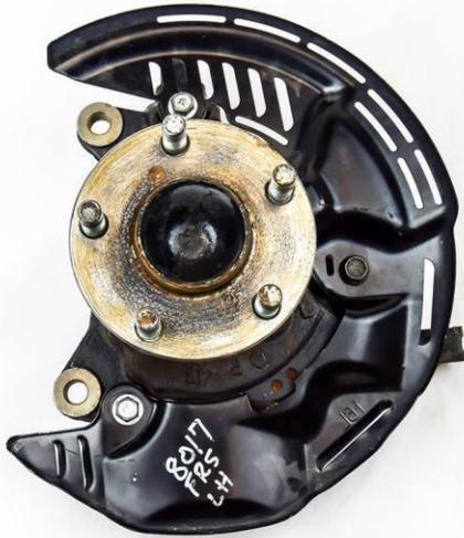
First start by removing your stock caliper and rotor until you are all the way down to the hub like shown in the first picture.
