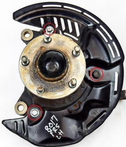
Next either remove your dust shield but taking out these three bolts circled in red. Or if you wish to keep it, simply trim the dust shield where it contacts your new rotor and caliper.
