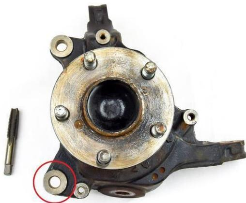
In this step you will take the included M14x2.0 tap and tap the bottom caliper mounting hole. This will hold your bracket stationary. If you do not wish to tap your spindle you can pick up a M12x1.25x55 bolt and a M12x1.25 nut to secure the bracket.
