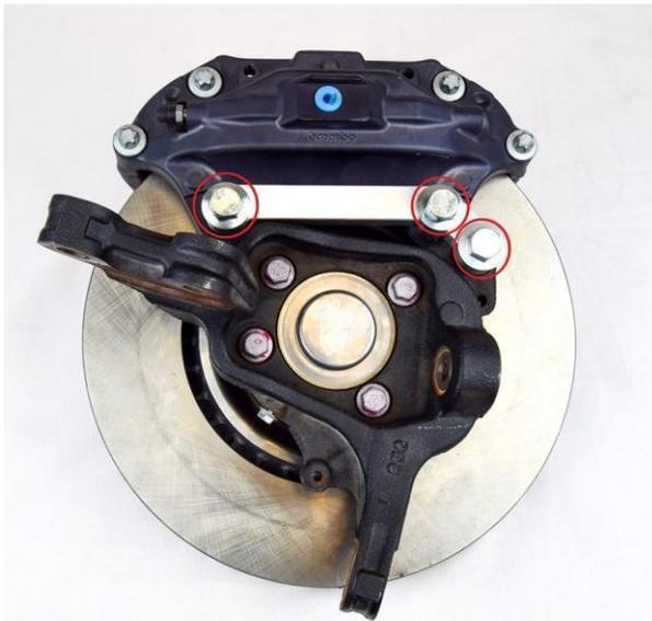
Next place the caliper on the bracket with the bleeders facing up. Begin to thread in the two longer M14 bolts supplied with the kit into the caliper as shown. Snug all three bolts evenly before tightening them all the way down.
