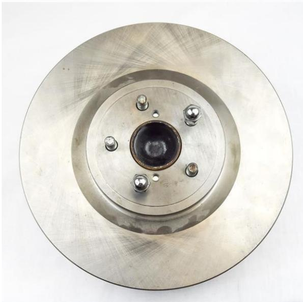
Next place the rotor on top of the spacer and screw on two lug nuts to keep the rotor secure.
