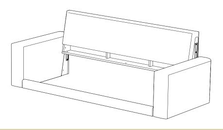
Make sure they are lined up before sliding the back piece down.
