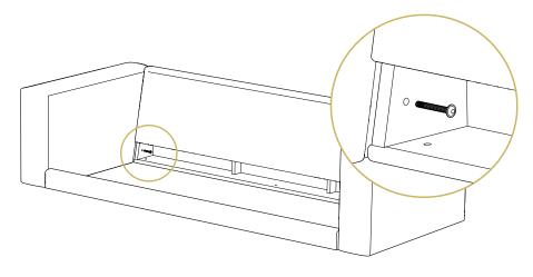
Tighten the bolt until firmly in place. Repeat with the other side of the front rail/arm.
