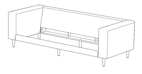
Platforms should lie at an angle, slightly raised in the front to ensure a comfortable seating pitch.
