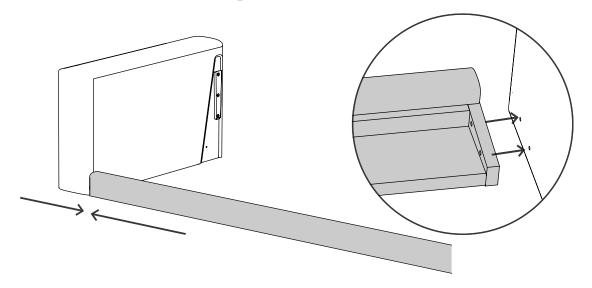
B Take 2 bolts and insert them into the holes in the front rail that lines up with the holes in the arms.
