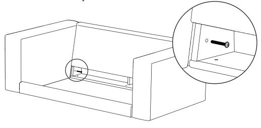
Tighten the bolt until firmly in place. Repeat with the other side of the front rail/arm.
