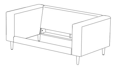
Platforms should lie at an angle, slightly raised in the front to ensure a comfortable seating pitch.
