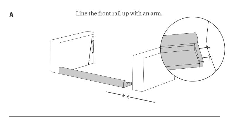
Take 2 bolts and insert them into the holes in the front rail that lines up with the holes in the arms.
