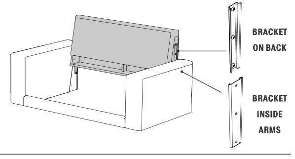
Make sure the brackets line up before sliding the back piece down.
