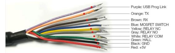
Purple: USB Prog Link, Black: GND, Red: +5V Connect usb programme linker TO pc/laptop for adjusting esc parameters
