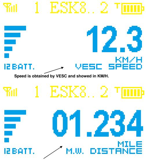
Distance is calculated based on RPM detected by one motor phase wire and showed in Mile.
