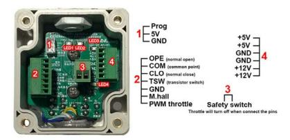
Wiring Pins Definition for MTSF300A-WP (with built in Maytech MTSRR1905WF receiver, can only work with Maytech remote)
