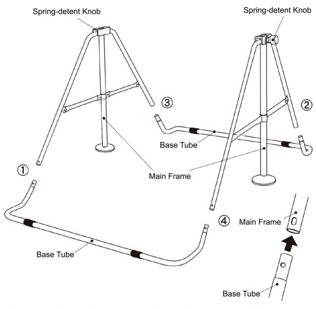
• Notice: Please let main frame and spring-detent knobs toward to outside, if not, the adjustable tube can't be install.
