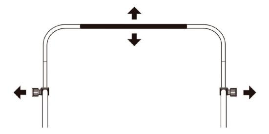
• Knobs: release two knobs, then pull it when the adjustable tube can be turned.
