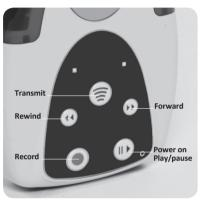
The remote control unit is an MP3 player, with an MP3 recorder, and has an infra-red wireless transmitter so that the teacher can collectively control the headphones. With this unit you are able to:
