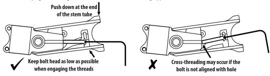
14. Approximately 32 turns are required to fully seat the preload wedge (#8). After about 5 turns, the preload bolt (#7) will require increasing torque to turn as the elastomers are compressed. Be sure to fully seat the preload wedge (#8) by applying 1.5 to 2.5 N-m of torque (use a torque wrench or tighten firmly using the short end of the included T25 Torx wrench as shown). Over-tightening may damage the preload wedge.
