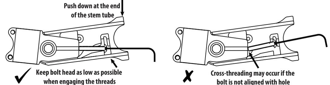
14. Approximately 32 turns are required to fully seat the preload wedge (#8). After about 5 turns, the preload bolt (#7) will require increasing torque to turn as the elastomers are compressed. Be sure to fully seat the preload wedge (#8) by applying 1.5 to 2.5 N-m of torque (use a torque wrench or tighten very firmly using the short end of a standard 3mm allen wrench as shown). Over-tightening may damage the preload wedge.
