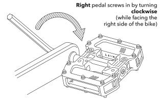
**CAUTION:** It's VERY IMPORTANT to correctly install the RIGHT vs. LEFT pedals. Incorrectly switching them and cross-threading will lead to damage! If the pedals are not going in easily by hand the first few turns make sure to check you have the correct pedal.
