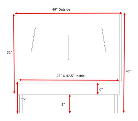
Available as Left, Right or center drain. 3.5" drain hole, located 7" on center from the left or right.
