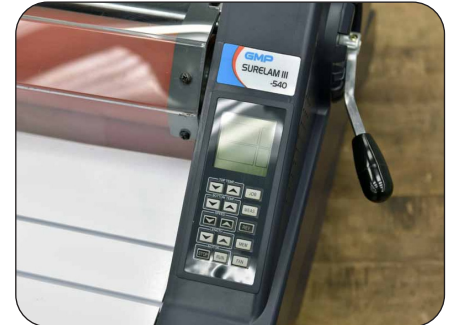
LCD control panel
