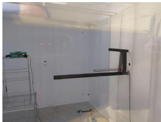
Fig. 6. Location of the ion counter in the chamber during the test which measured the level of negative ions in the chamber
