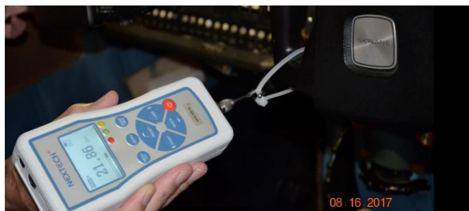
FIGURE 5-3 ELEVATOR HELD IN NEUTRAL POSITION USING FORCE GAUGE
