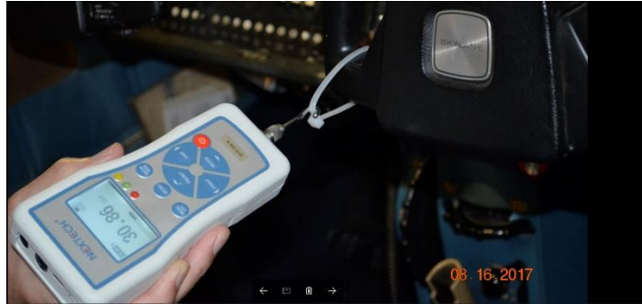
FIGURE 5-4 FORCE GAUGE USED TO OVERRIDE V NAV SERVO
