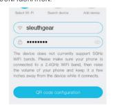
3g. A QR code will display on the smart phone screen. Use the camera to scan the QR code 4" away from the smart phone screen
