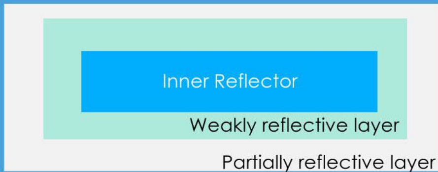
Figure 3. Cross section of an optically variable (ColorShift) pigment. Certain colors are reflected while others are transmitted.
