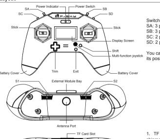
SA: 3 positions; Long lever SB: 3 positions; Long lever
