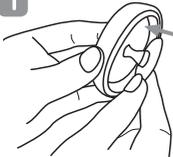
Insert the stem into the diaphragm.
