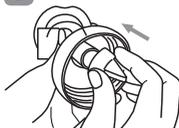
Hold the base of the silicone valve and attach it to the main body.
