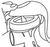
Press the "PUSH" part at the tip of the handle to set the handle hole into the first (top) notch of the stem.
