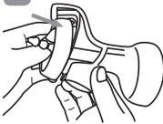
Place the diaphragm on top of the main body. Firmly seat the bottom of the diaphragm in the groove of the main body. If not fitted securely, air will leak through and the pump will not be able to achieve suction.
