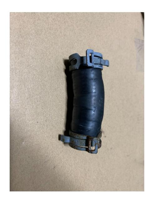
1.2: This is the factory hose that runs under the frame rail that is removed and capped. We will be removing the hose pictured here and it will not be re-used.
