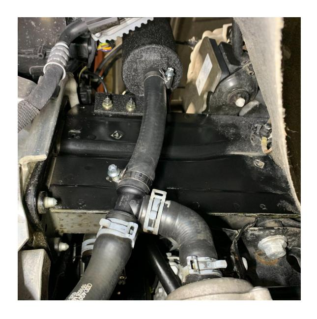
1.4: Install the hose to the bottom of the coolant reservoir, lubricate and install the bottom of the hose to the factory coolant tee, and install the bracket to the frame studs using the included nuts and washers.
