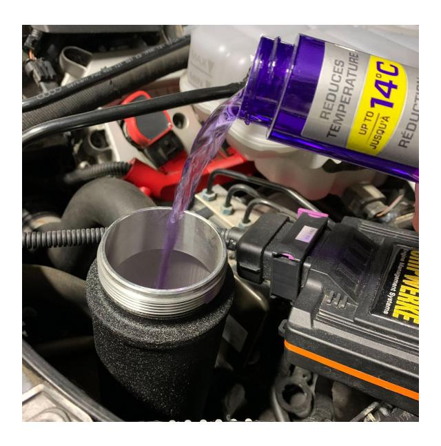
1.6: Fill the reservoir with 50/50 G13 coolant mix, or a bottle of Royal Purple "Purple Ice". Do *not* use universal coolants or Redline "Water Wetter", as these are not compatible with VW's G13 coolant.
