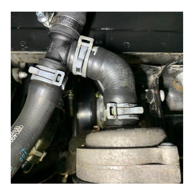
1.3: The tee shown here will have to be re-positioned so that one leg is pointing upwards (as shown in this image) to allow for installation of the coolant reservoir.
