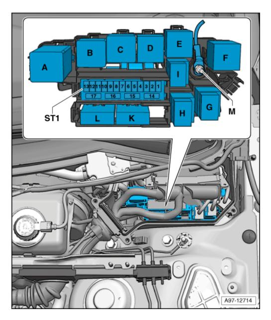
**SA16** - Fuse #16 in carrier ST1 (**A**) in the underhood fuse panel SA Location: Under washer fluid filler neck
