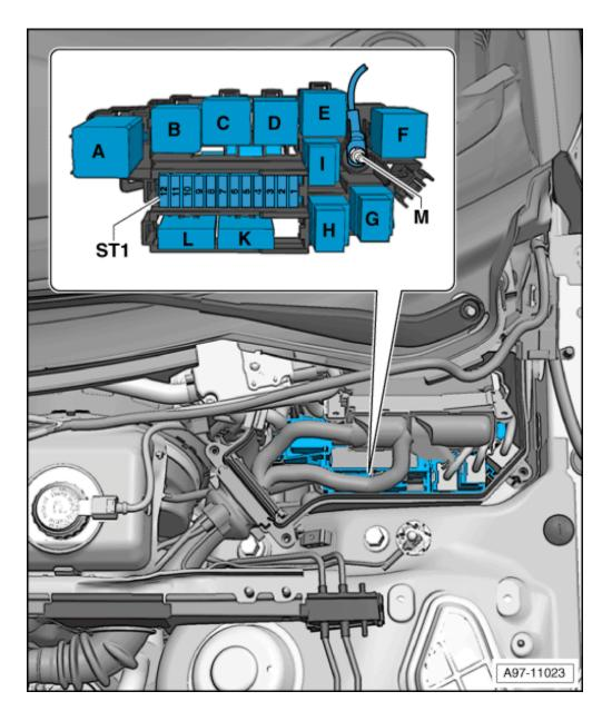
**SB16** - Fuse #16 in carrier ST1 in the underhood fuse panel SB Location: Under washer fluid filler neck
