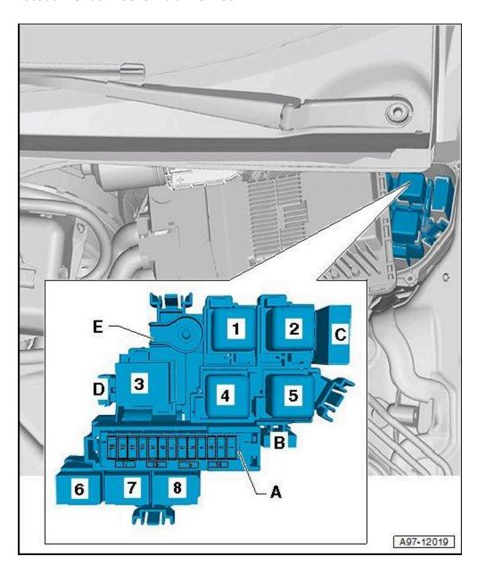
**SA10** - Fuse #10 in carrier ST1 (**A**) in the underhood fuse panel SA Location: Under washer fluid filler neck
