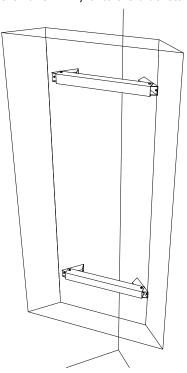
For horizontal mounting of tiles and traps where the wall meets the ceiling, use our "Corner Bracket Wall:Ceiling" system.
