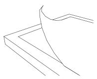
Remove the self adhesive backing from the Stick Pins and apply them to the wall, positioning them according to the panel size and desired orientation at least 100mm from the panel edges.
