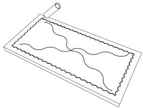
Align the panel accurately then carefully but firmly press the panel into position.
