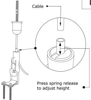
Ensure distance between fixings is always under 1m to provide adequate support for the panel
