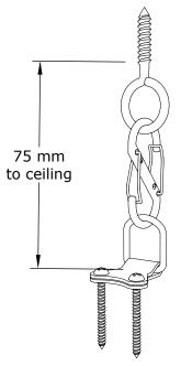
Position panel hanger mounts 80mm in from panel edges
