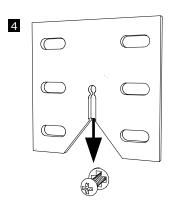
Slide the panel onto the Centre Screw until all Flexi Clips lock
