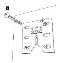
Secure Flexi Clips to panel using EQ\_Fibre Screws.
