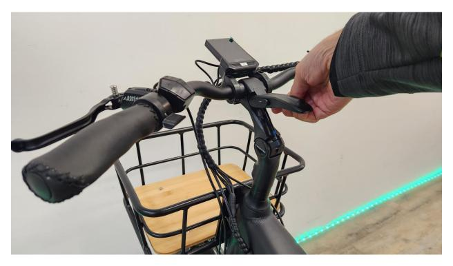
Photo A – Handlebar Lock Lever in Open and Unlocked Position
