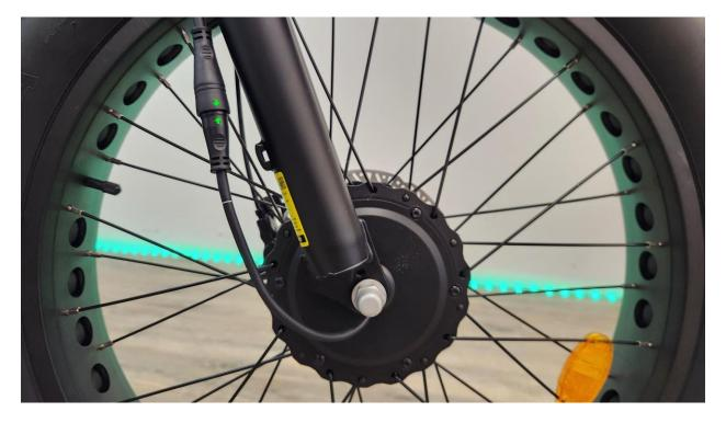
Line up the arrows on the motor connection cable and plug firmly together until they snap into place.
