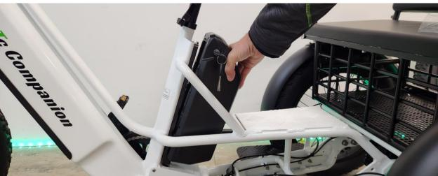
Line the tabs on the battery (red arrows) with the notches on the battery mount on the frame (green arrows) Then carefully push down firmly until the battery snaps into place.
