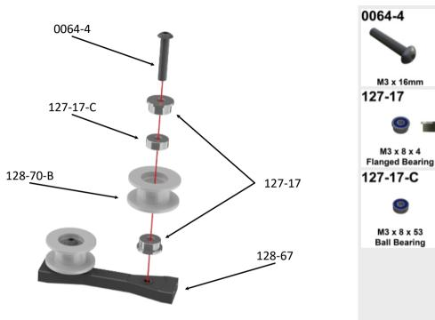
Apply a small amount of medium thread lock when threading in to metall parts.
