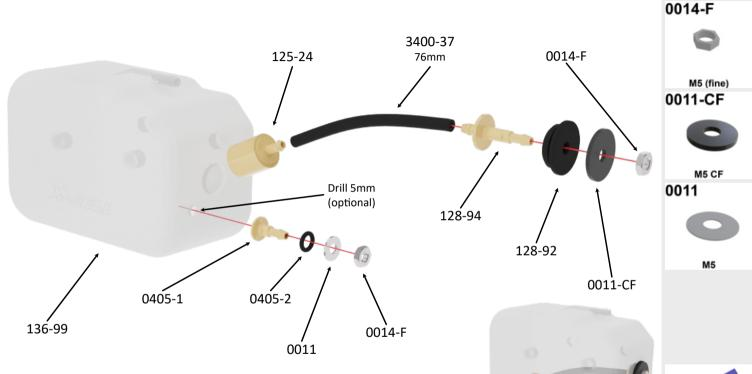
Assembly Tip: Do not apply thread lock to the nut 0014-F. Do not overtighten. If the tank starts leaking at this opening just tigthen the nut about 1/2 or 1 turn.
