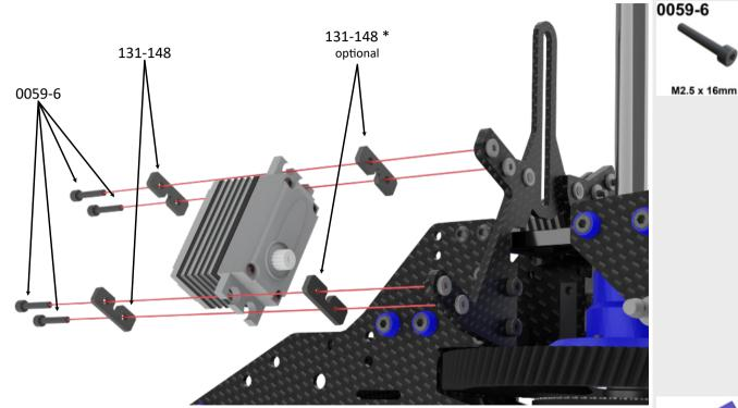
\* MA128-172 Servo Spacers are included for proper servo linkage alignment, if required.
