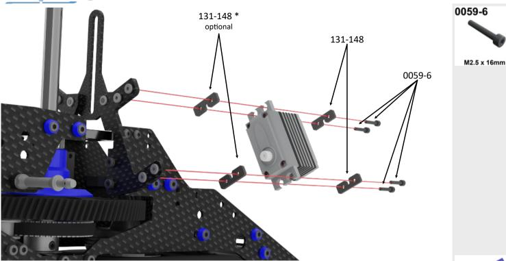
\* MA128-172 Servo Spacers are included for proper servo linkage alignment, if required.
