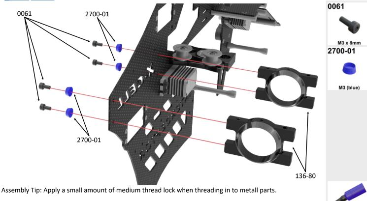
Apply a small amount of medium thread lock when threading into metal parts.
