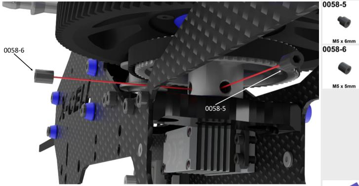
Assembly Tip: Take care that the dog point socket set screw 0058-5 will settle at the dimple of the main shaft. Tighten this screw first.
