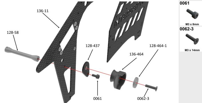
Assembly Tip: Align the opening of part 136-464 to the front of the helicopter.
