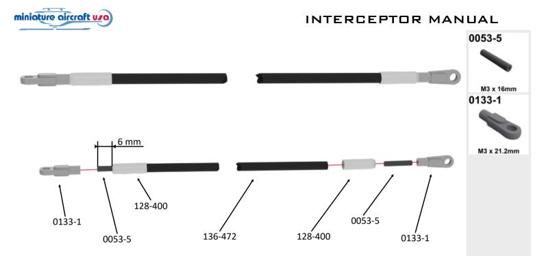
Assembly Tip: Install the 0053-5 set screws into the push rod ends use high quality epoxy. Put all parts together and check length of the push rod. Shorten carbon tube is nescessary. Use some high quality two-component epoxy to glue the push rod ends to the carbon tube. Put epoxy at the inside and the outside of the carbon tube to glue the push rod ends at it.
