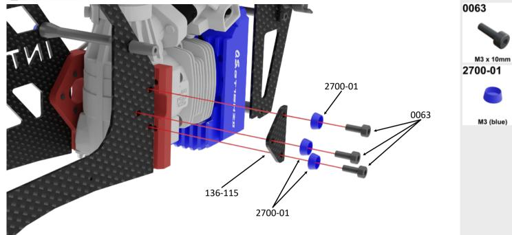
Assembly Tip: Apply a small amount of medium thread lock when threading in to metall parts.
