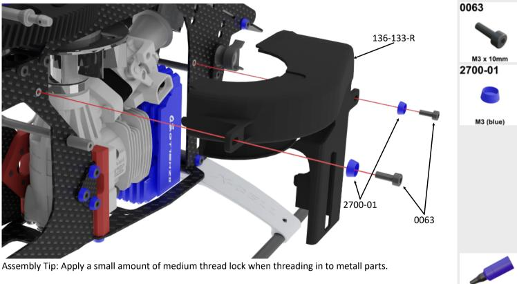
Check that fan shroud left and right it together.
