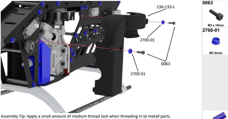
Check that fan shroud left and right it together.
