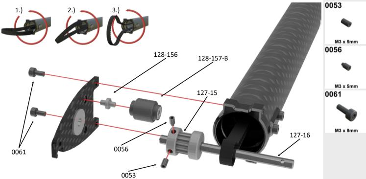
Assembly Tip: Apply a small amount of medium thread lock when threading in to metall parts. Attention: Turn the belt 90 degress counter clockwise.
