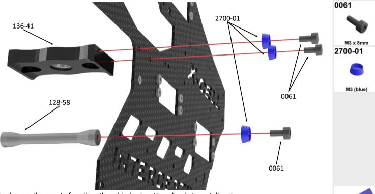
Apply a small amount of medium thread lock when threading in to metall parts.
