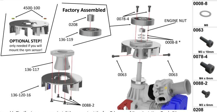
Assembly Tip: If using a governor install the magnets at the fan. Take care of the orientation. On shall be facing up "North" the other shall be facing up "South". Use some high quality two-component epoxy like UHU 300 and let it hardening. The magnets are included in the Interceptor kit. \* 0008-8 second is optional
