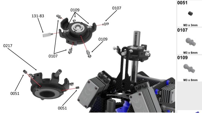
Thread in the MA0051 m3x3 socket set screwsinto the base of the swashplate only until they bottom out against the lower bearing.
