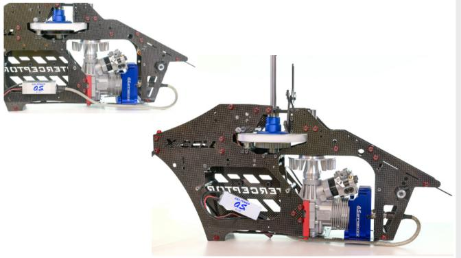
Assembly Tip: The ignition box will be mounted on the bottom platte using a thin douple sided adhesive tape.
