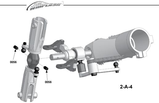
Apply a small amount of medium thread lock when threading into metal parts
