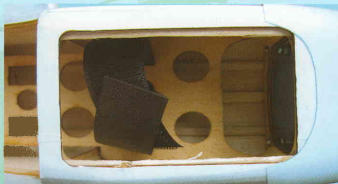
11B- Battery location
