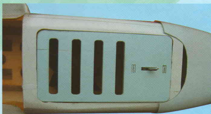
11A- Battery hatch installed
