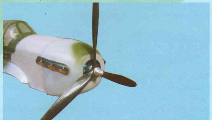
10E- Install the suitable propeller and spinner
