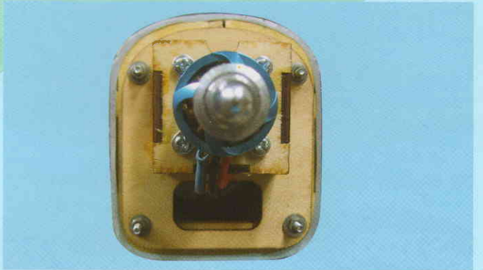
9D- Secure power module to the fuselage by using 4 sheet metal screws 2 x 10mm
