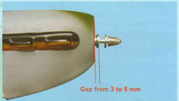
10C- Trial fit cowl to the fuselage
