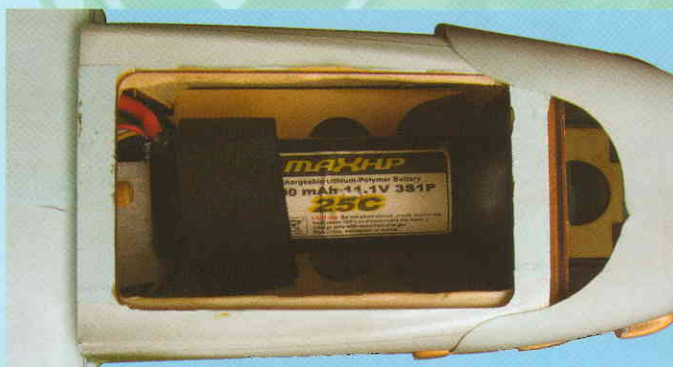
11A- Battery installed
