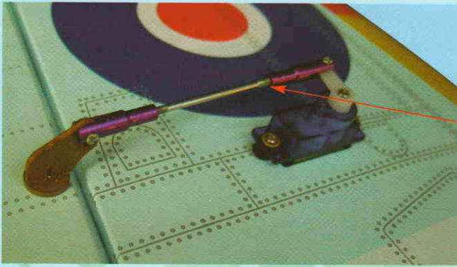
1G- Connect the aileron control rod one end to the servo arm and other end to the control horn
