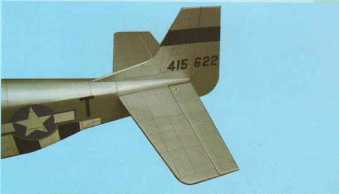
4A- Trial fit the vertical stabilizer to the vertical slot
