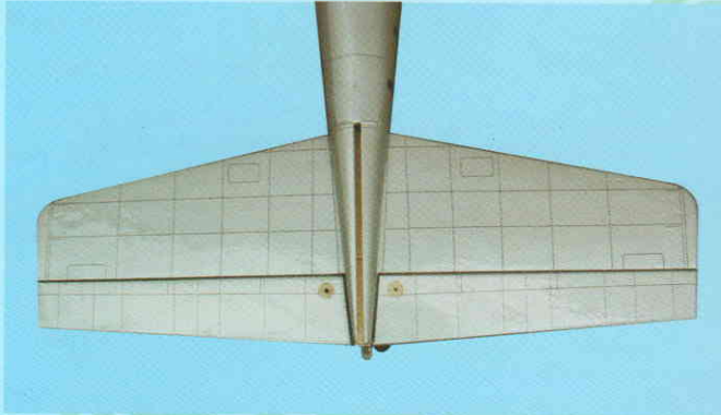
3A- Trial fit the horizontal stabilizer to the fuselage
