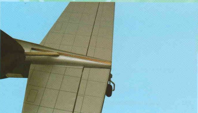
4C- Apply sufficient 30 minute epoxy to the vertical slot
