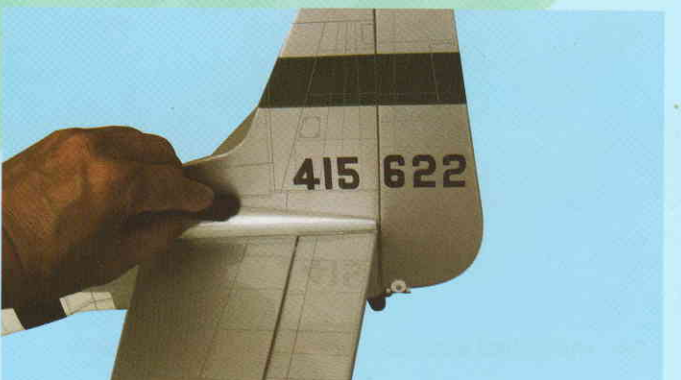
4D- Insert the vertical stabilizer into the slot, then wipe off the excess epoxy
