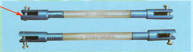
1H- Aileron control rod assembly
