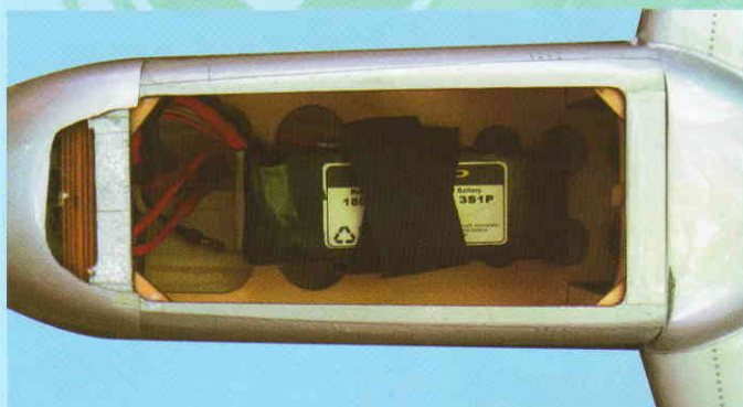
11A- Battery installed
