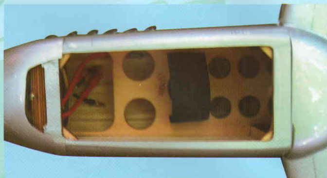
11B- Battery location
