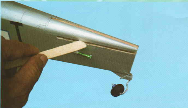
3C- Apply sufficient 30 minute epoxy glue to the horizontal slot
