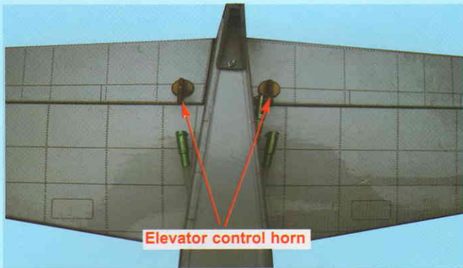
7C- Elevator control horn mount to the elevator
