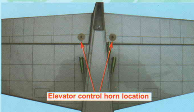
7A- Elevator control horn location
