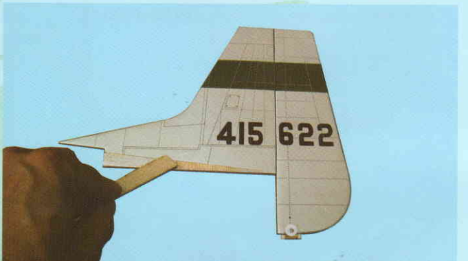
4B- Apply sufficient 30 minute epoxy to the expose wood area on both side of the vertical stabilizer
