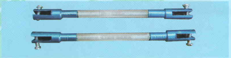
1A - 2 aileron control rods assembly
