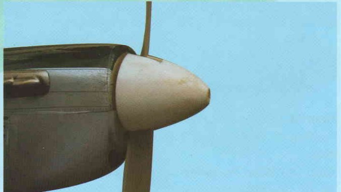
10F- Install the suitable propeller and spinner
