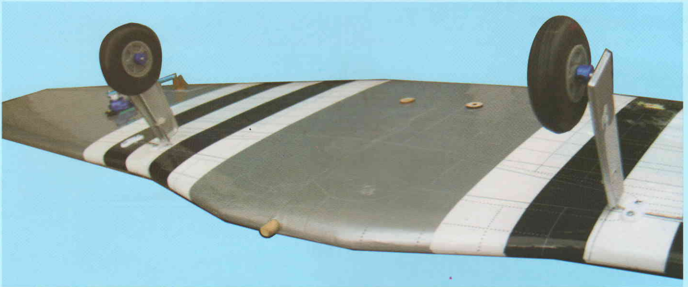
5E- The 2 main landing gear mount onto the wing
