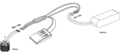
1). Plug the programming cable (on your ESC) into the programming port on the LED program box. Note: Need plug the throttle signal cable into the power port on the LED program box and the programming wire (yellow wire) into the programming port on the LED program box.
