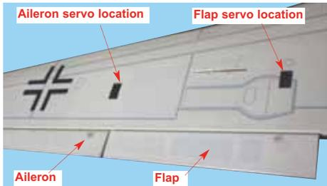
4B - Location of aileron, aileron servo, flap and flap servo
