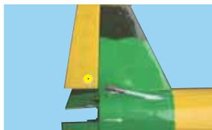
12B- Rudder control horn location
