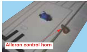
5B- Aileron control horn and servo installed
