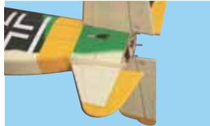
8F- Trial fit the bottom vertical stabilizer into bottom slot
