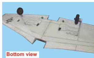
9C- Both main landing gear mounted to the wing
