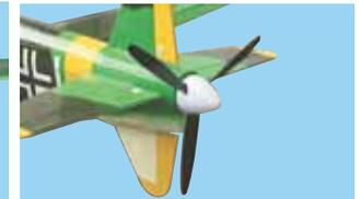
11H- Cowl,propeller and spinner installed to the rear end
