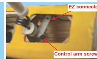
10B- Insert the nose gear steering control arm to the EZ connector then insert the nose gear assembly into the nose gear bearing then tighteng the control arm screw
