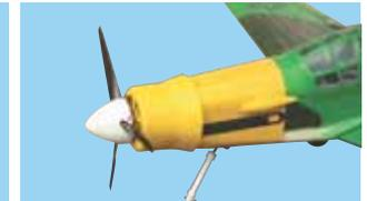
11H- Cowl,propeller and spinner are installed to the nose
