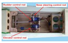
13B- Elevator servo connected to the elevator control rod,rudder servo connected to the rudder and gear steering control rod
