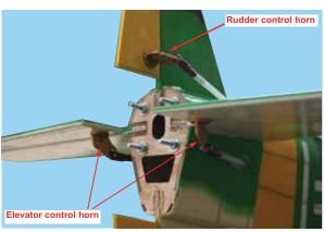
12C- Elevator control horns and rudder control horn installed in its location and connected to the clevises
