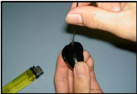
6. BIND COVER AND BOTTOM OF SPINNER. DRILL RIGHT AND LEFT SIDE FOR 2.3X6 TAPPING SCREW.
