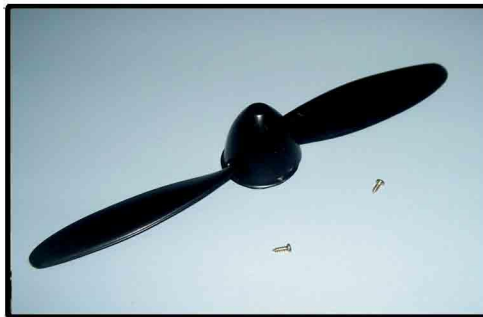
7. TRY TO PUT PROPELLER TO SPINNER. CHECK IF FIT AND TRIM.
