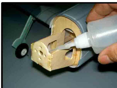
1. FIX MOTOR MOUNT PLYWOOD INTO FIREWALL WITH CA GLUE.
