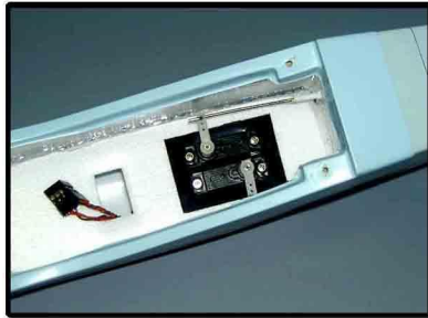
4. INSTALL THE RUDDER PUSH ROD TO RUDDER SERVO HORN. INSTALL THE ELEVATOR PUSH ROD TO ELEVATOR SERVO HORN.
