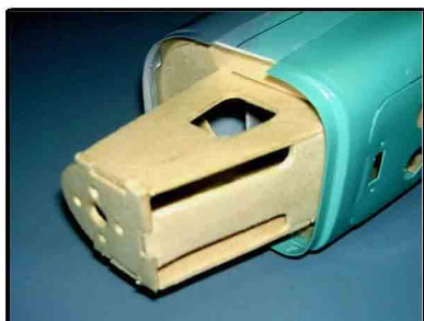
1. FIX MOTOR MOUNT PLYWOOD INTO FIREWALL WITH CA GLUE.
