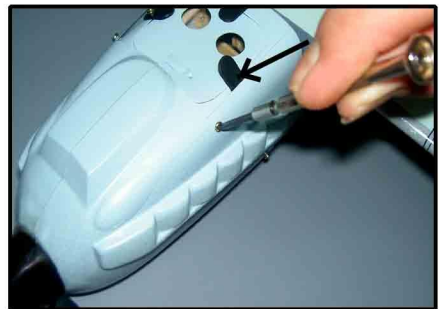
13. DRILLING HOLES. USE TAPPING SCREW 2. 3X6. FIX BATTERY COVE STOPPER. INSTALL THE BATTERY
