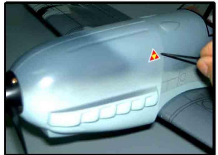
11. CHECK THE FIT OF SPINNER AND COWLING. LEAVE ABOUT 1.5mm GAP TO AVOID INTERFERENCE. DRILL 4 HOLES ON COWLING AND PLASTIC FUSELAGE
