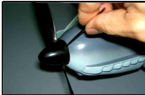
10. FIX SPINNER WITH 2.3X6 TAPPING SCREW.
